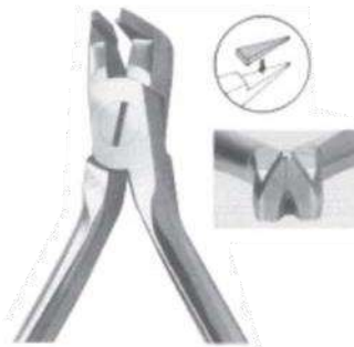
61-4022-TC Distal End Safety Cutter Maximum Cutting Capacity ■ Rectangular Wires up to .022 x .028" ● Round Wires up to .020" ▼ Brided Wires up to .016"
